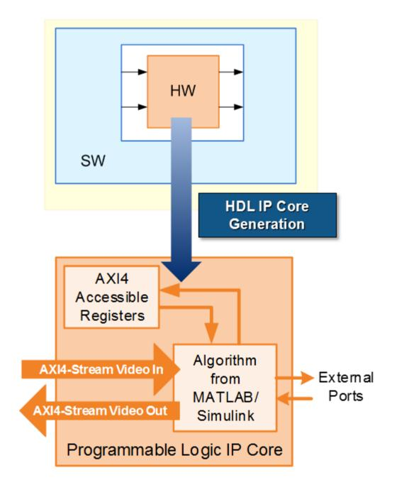
**3** *Embedded System Tool Integration*: As part of the HDL Workflow Advisor IP core generation workflow, you insert your generated IP core into a *reference design*, and generate an FPGA bitstream for the SoC hardware.
