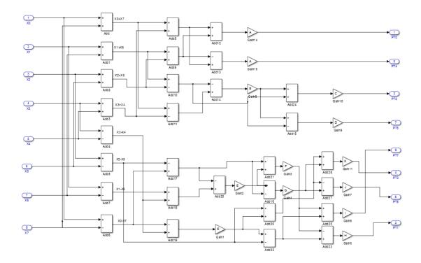
Set **DistributedPipelining** to **off** and **OutputPipeline** to **6** to insert 6 pipeline stages at the outputs of the DUT.
