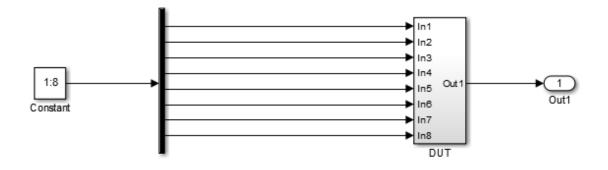
The top-level subsystem is the design under test (DUT). The DUT subsystem contains one subsystem, subsys, and other blocks.
