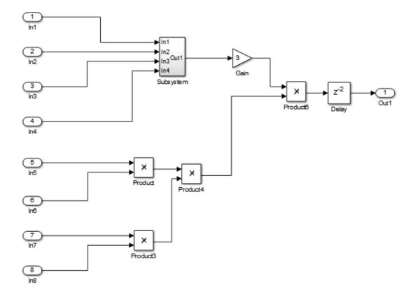
The following diagram shows the model after applying hierarchical distributed pipelining:
