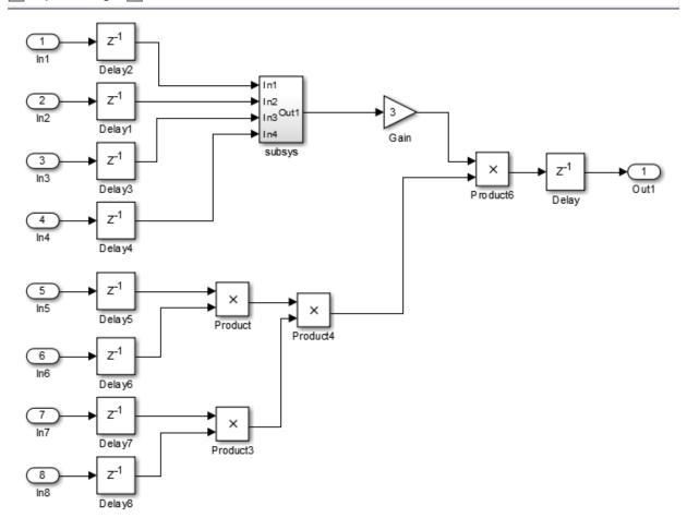
The subsys block in DUT contains a copy of the three Product blocks in the lower half of the diagram.
