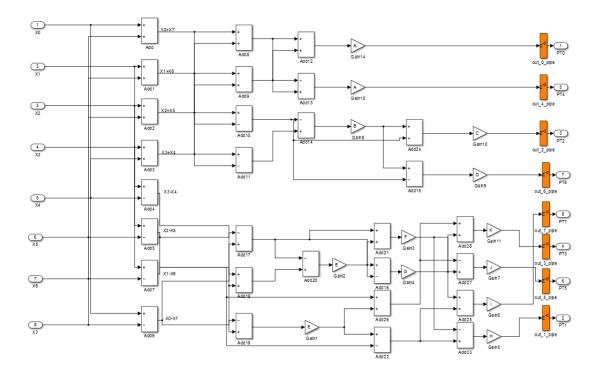
Set **DistributedPipelining** to **on** and **OutputPipeline** to **6** to distribute 6 pipeline stages for each signal path in the DUT.
