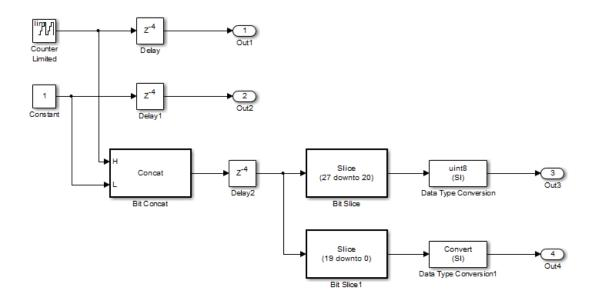
The Delay and Delay1 blocks merge and map to a dual-port RAM in the generated HDL code by satisfying the following conditions:
