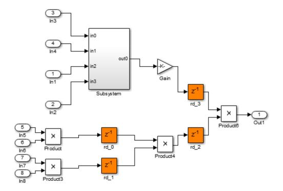
The subsystem now contains pipeline registers:
