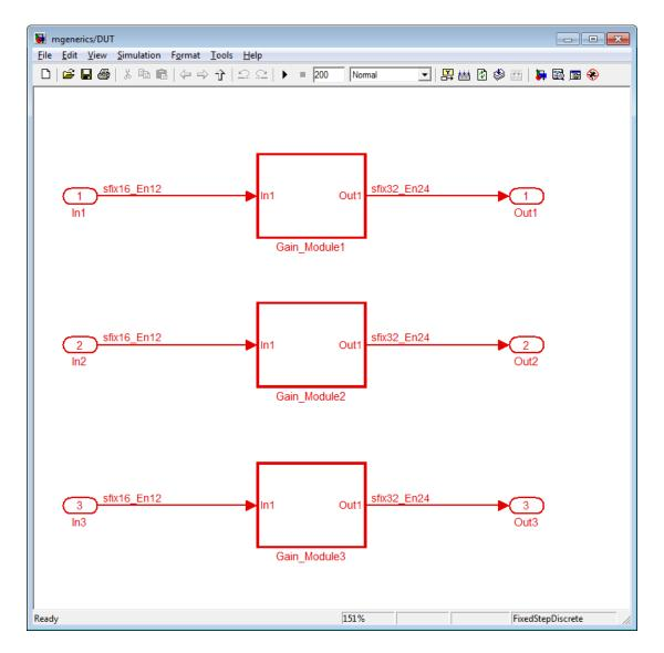
In mgenerics/DUT, the gain modules are subsystems with gain values represented by tunable mask parameters. Gain values are 0.6 for Gain\_Module1, 2.4 for Gain Module2, and 6.8 for Gain Module3.
