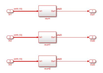
The DUT subsystem contains three subsystems that are identical except for their subsystem names.
